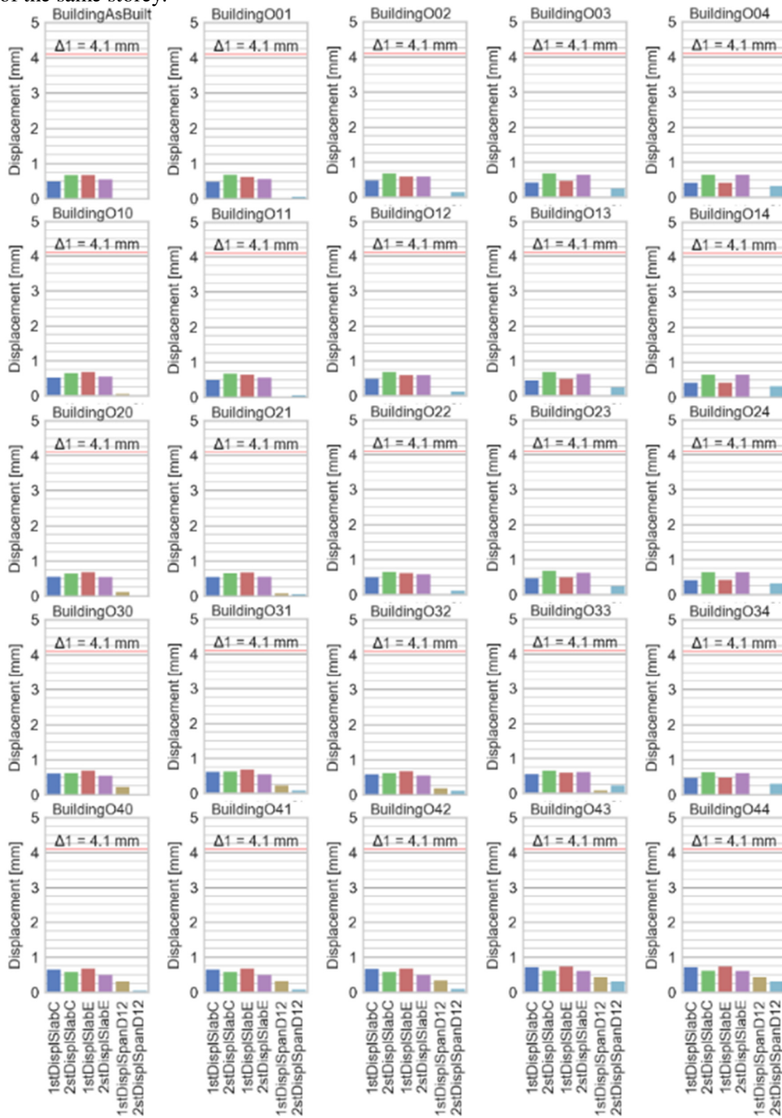
Figure 25 Variation of vertical deflections of slabs and spandrels relative to allowable deflections
