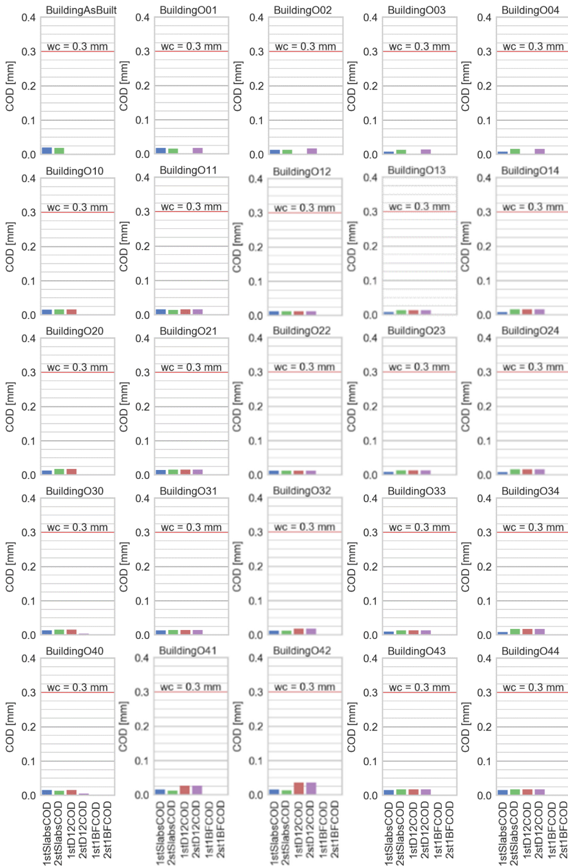
Figure 26 Variation of maximum crack opening displacements (COD) relative to allowable crack openings ( w_c )
